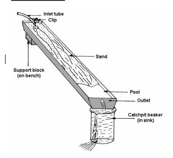
You need a 1m (approx) length of gutter with two stop ends. This should be filled about <sup>2</sup>/<sub>3</sub> full of damp sand (e.g. washed builders' sand) along about <sup>3</sup>/<sub>4</sub> of its length. Mount one end on a wood block (or similar), with the other end over the sink. It is a good idea to drill an outlet hole in the lower end-stop; a beaker in the sink can also provide a catch-pit for any escaping sand.
