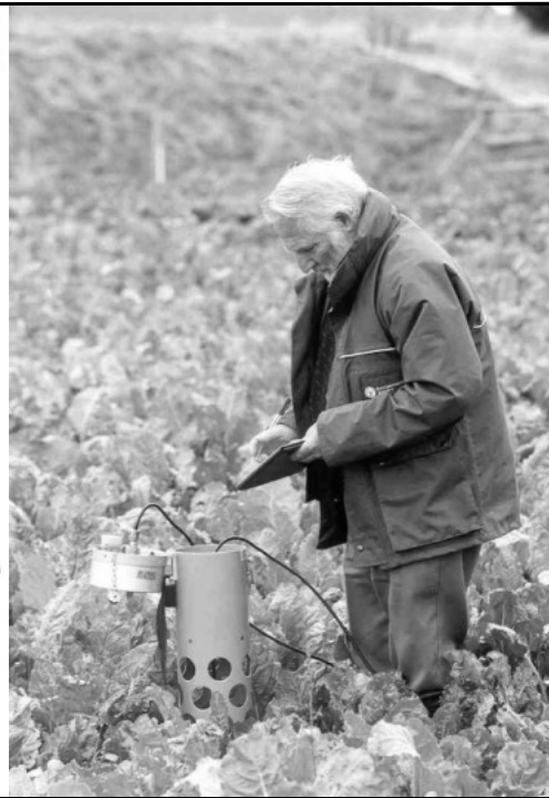
The Principle of the Neutron Soil Moisture Probe Fig.A.5.1.
